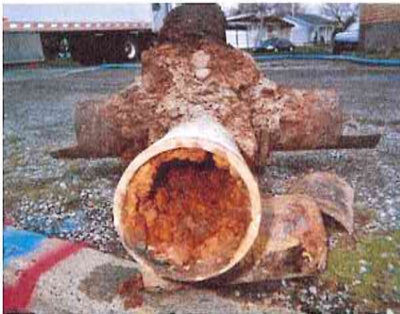
Figure 9: Water Main Before Cleaning
