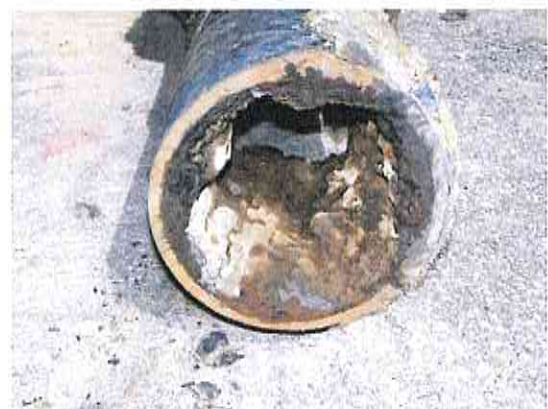
Tuberculation in the existing water pipe led to decreased water pressure along 4th street.
